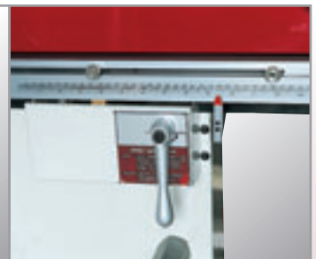
Crossfeed lock and proximity switch design for crossfeed travel. (Model 1020 & above)
