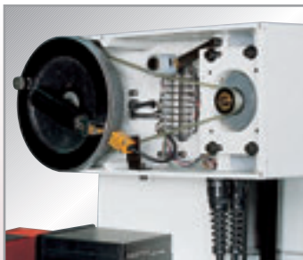
Stepping motor on downfeed system ensures an accurate downfeed amount. (Model 818)
