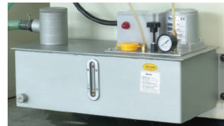
Automatic lubrication pump with re-circulating system.
