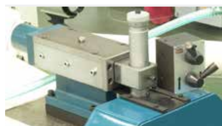
Hydraulic over-head wheel dresser.
