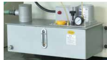
Automatic lubrication pump with re-circulating system.
