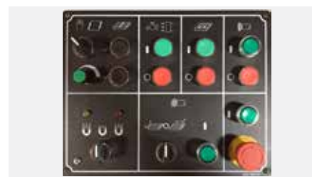
Automatic plunge and surface grinding modes, AHD models.
