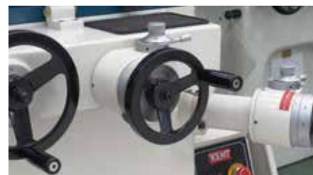
Micro 0.00005" down-feed and cross-feed devices, for 616 model.
