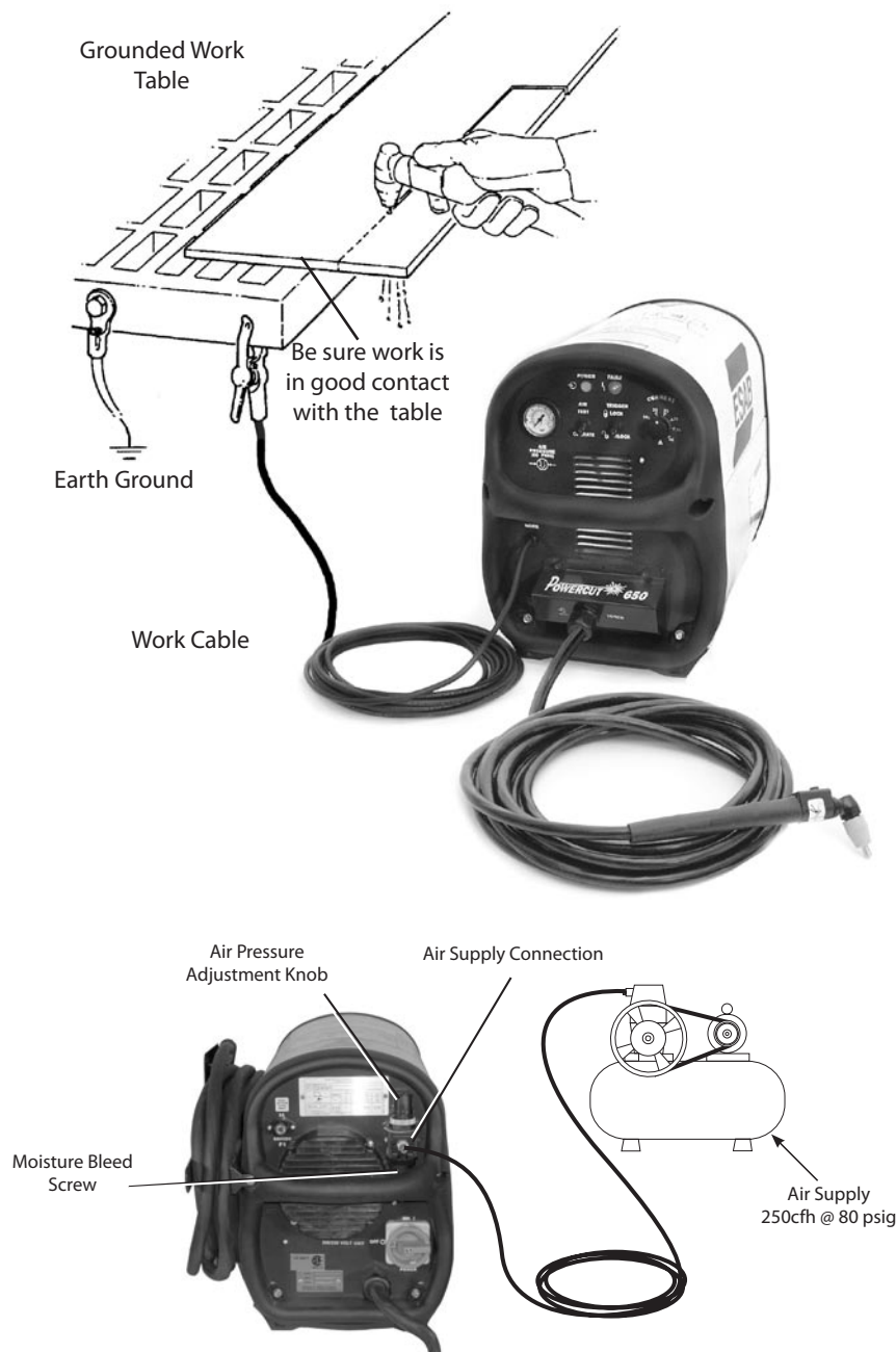
Figure 3.3 Secondary Connections Diagram
