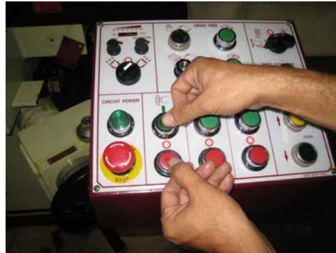
Fig. 4 Push On and Off immediately. Make sure spindle rotation is clockwise.
