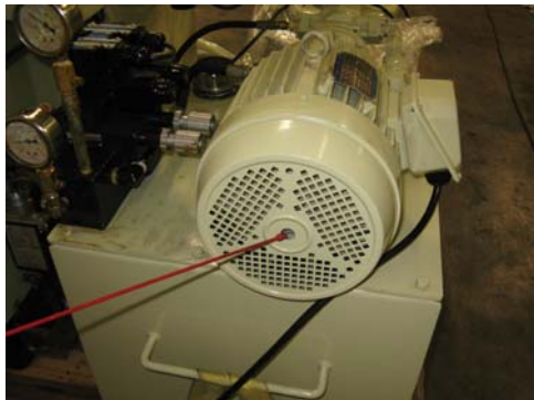
Fig. 5 Make sure hydraulic motor rotation is clockwise.
