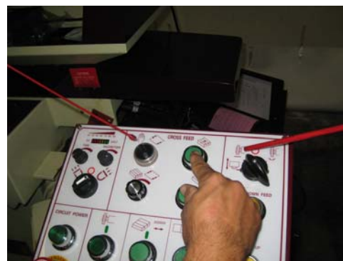
Fig. 9 Make sure Rapid Up/Down direction is correct. Make sure Function Switch on Rapid Mode.
