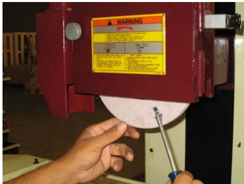
Fig. 3 Tap wheel with object to make sure wheel is not cracked. The sound should be clear and consistent.
