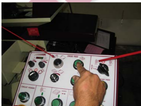
Fig. 8 Make sure Rapid Up/Down direction is correct. Make sure Function Switch on Rapid Mode.
